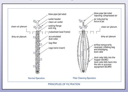
The Dalamatic® system uses an envelope-shaped filter bag and pulses of air to provide greater movement of the bag to dislodge more challenging dust cakes during filter pulsing. The dislodged dust cake falls into the collection hopper for final removal or is routed directly back into the process.
